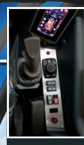
Pressurized cab ISO 10.263 Standard air conditioning and heating Touch screen display with joystick control system
